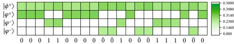
FIGURE 5: A stream of random numbers obtained by retrieving the King’s measurements. In a game between Alice and the King, after the initial state  $|\phi^+\rangle$  is distributed, a series of  $b$  values are randomly chosen by the King and the corresponding nonselective measurements in MUBs are implemented successively. Then Alice can “guess” the King’s choice by her own measurement. The measured probabilities are represented by the color, and the identified random numbers are listed below.
