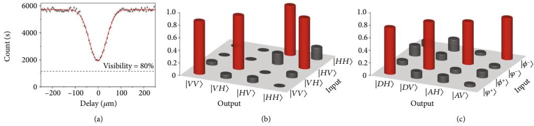
FIGURE 3: The complete characterization of the control measurement system. (a) By injecting the state  $|H\rangle_a|H\rangle_b$ , the two-photon interference is shown via the Hong-Ou-Mandel dip with the obtained visibility of 66.3%. (b) The truth table measured in the computational basis  $ZZ$ . (c) Demonstration of the ability of the C-NOT gate to transform the maximally entangled states into corresponding product states.
